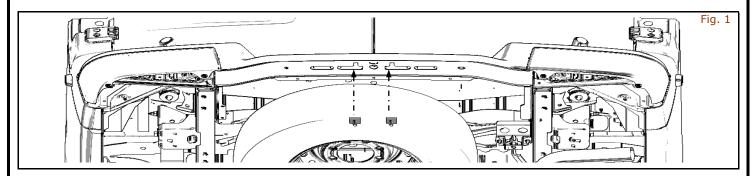
2) Install Bolt Stud on bottom of rear bumper (2 places)
