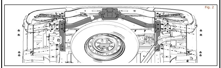
3) Raise Hitch into vehicle position and install bolt (8 places)
